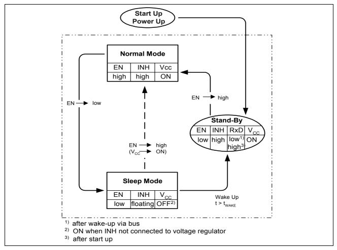
Figure 3: operation mode state diagram
