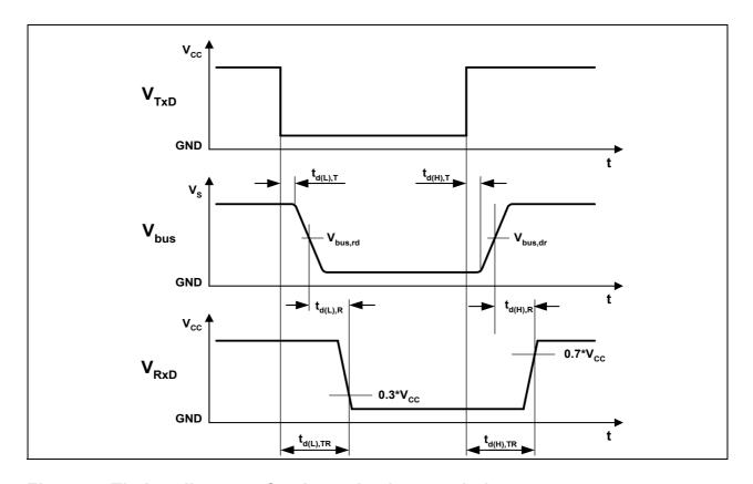
Figure 5: Timing diagrams for dynamic characteristics
